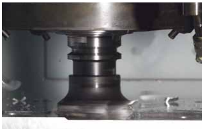
Cutting with NSK spindle using ceramic ball bearing
